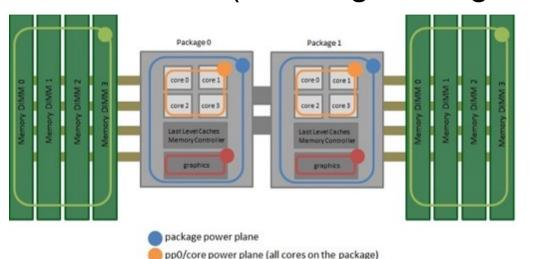
Energy measurements: PACKAGE ENERGY: PACKAGEO 176.450363J (Average Power 42.9W) PACKAGE ENERGY: PACKAGE1 75.812454J (Average Power 18.4W) 11.899246J DRAM ENERGY: PACKAGEO (Average Power 2.9W) DRAM ENERGY: PACKAGE1 8.341141J (Average Power 2.0W) PPO ENERGY: PACKAGEO 118.029236J (Average Power 28.7W) PPO ENERGY: PACKAGE1 16.759064J (Average Power 4.1W)
